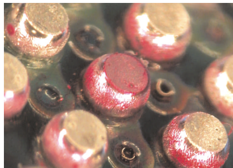
FIGURE 5. Liquid dye placed between this BGA and the PCB it was soldered to penetrated a space that existed between the center solder ball and its solder pad. The other balls were soldered properly to their respective pads, so no dye penetrated these junctions.
