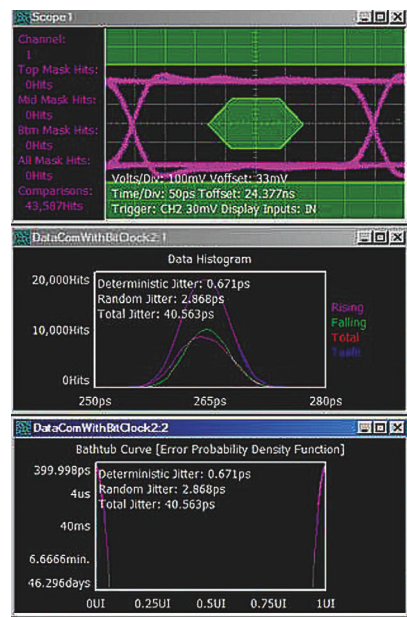
FIGURE 2. An eye mask (top) enables go/no-go testing, while a histogram (middle) indicates the jitter of rising and falling data edges relative to the clock signal. The bathtub curve data enables derivation of DJ, RJ, and TJ values using a tail-fit algorithm.
